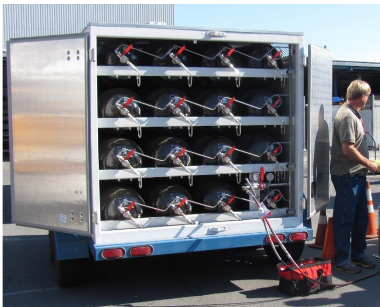
Figure 3.1: IGX 350 bar refueling trailer in use at the San Francisco International Airport to refuel hydrogen fuel cell mobile lights, July 23, 2013. Photo Credit: Lennie Klebanoff.
