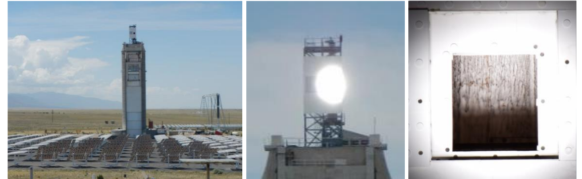
On-sun testing of the falling particle receiver at Sandia
