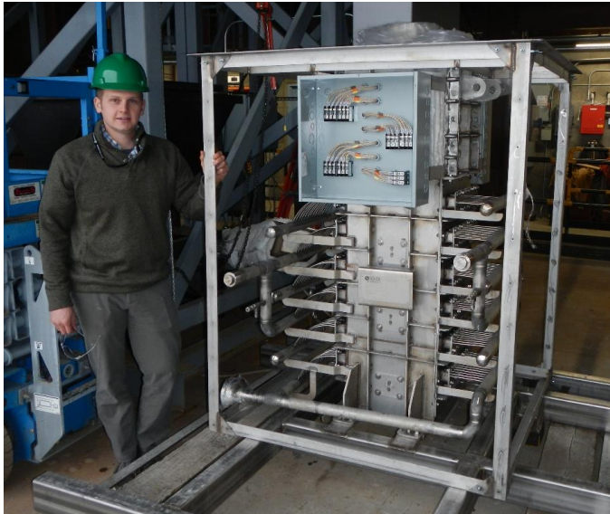
100 kW particle-to-sCO 2 heat exchanger
