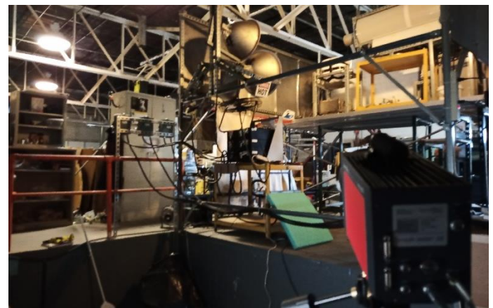
Figure 3. InfraTec thermographic system ImageIR® 8320 HP with 100 mm lens is used to record the thermograms from the SPR from the front view.
