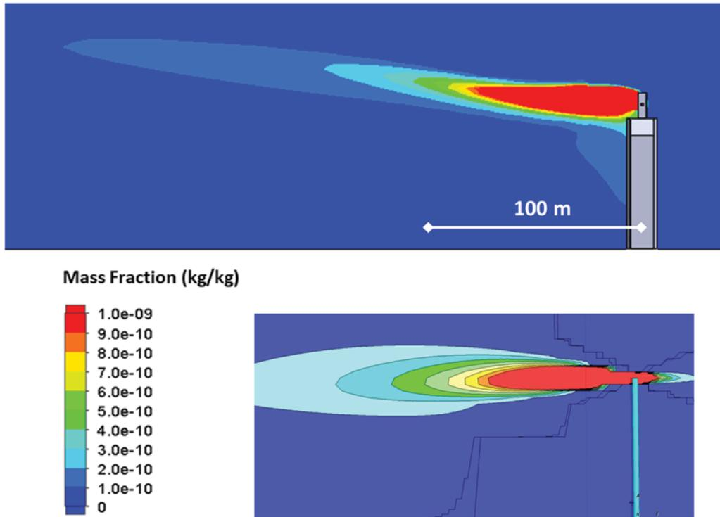
**FIGURE 3.** Simulated small particle ( $<10 \mu\text{m}$ ) mass fractions in air with a west wind speed of 2 m/s using CFD (top) and AERMOD (bottom).
