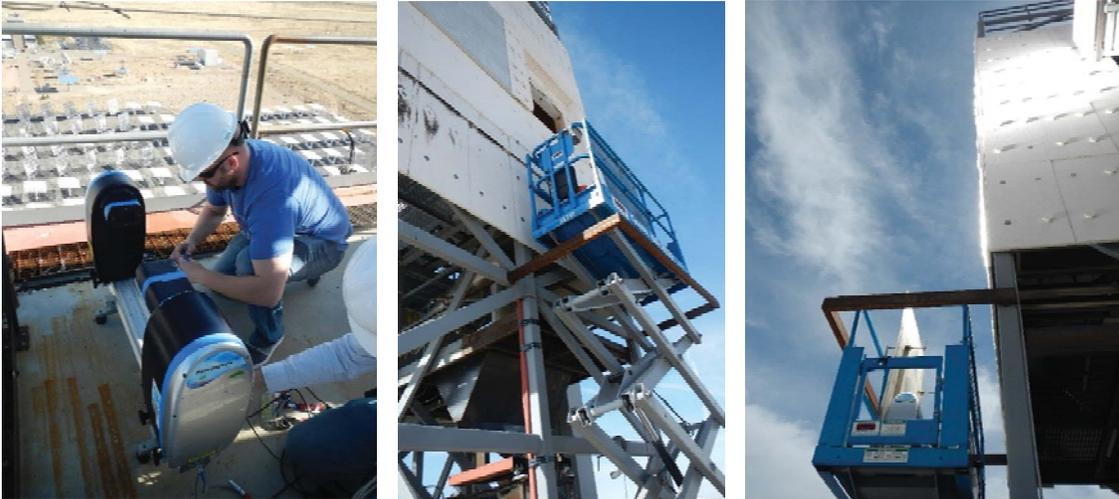
**FIGURE 1.** Images of the Malvern Spraytec used to evaluate large particle emissions (tens to hundreds of microns) at the NSTTF. The Spraytec was placed in an aerial lift to be positioned just beneath the aperture of the receiver [7].
