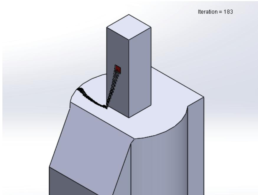
**FIGURE 4.** CFD simulation of 350  $\mu\text{m}$  particles emitted from receiver aperture at the NSTTF (0.003 kg/s, 2 m/s west wind).
