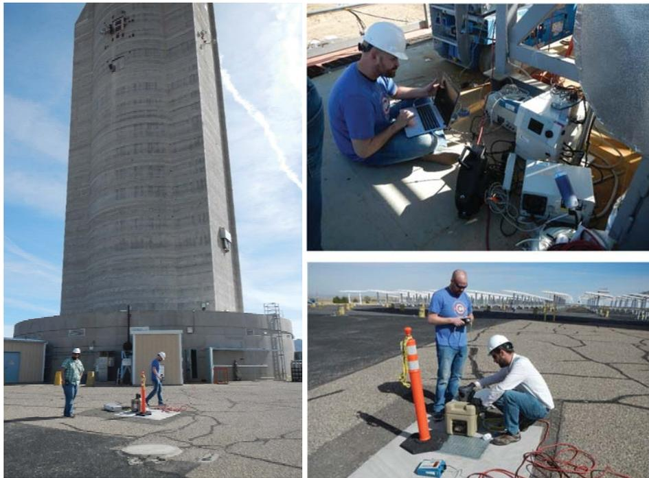
**FIGURE 2.** Traditional volumetric air samplers were used to evaluate small particle emissions (submicron to micron) at the base and top of the tower at the NSTTF [7].
