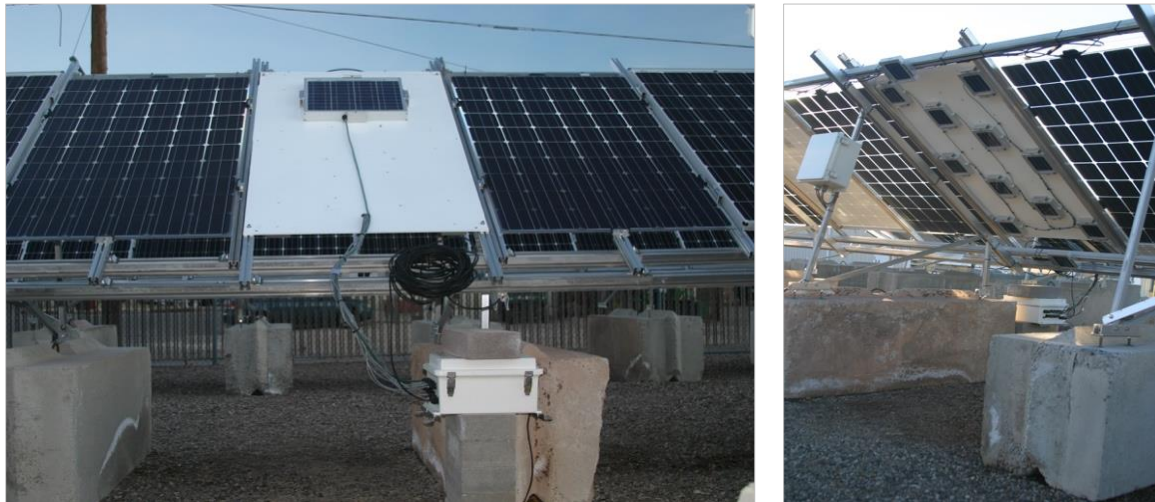
Figure 21: (left) Front side of the IDM placed in the middle of a row of modules. (right) Back side of the IDM.
