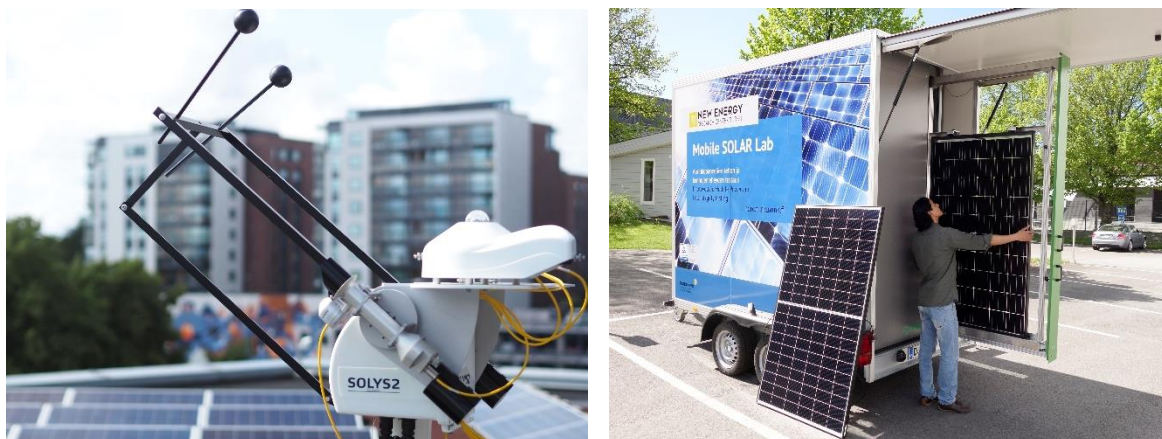
Figure 112: (left) Solar irradiance monitoring, including diffuse horizontal irradiance (DHI), direct normal irradiance (DNI), mounted south of tracker. (right) Modules are characterized by triple A+ Mobile Solar Simulator.
