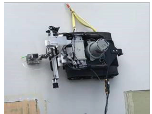
Sandia ARROW(e) Inspection Robot. Image Credit: Sandia, Dennis Roach
