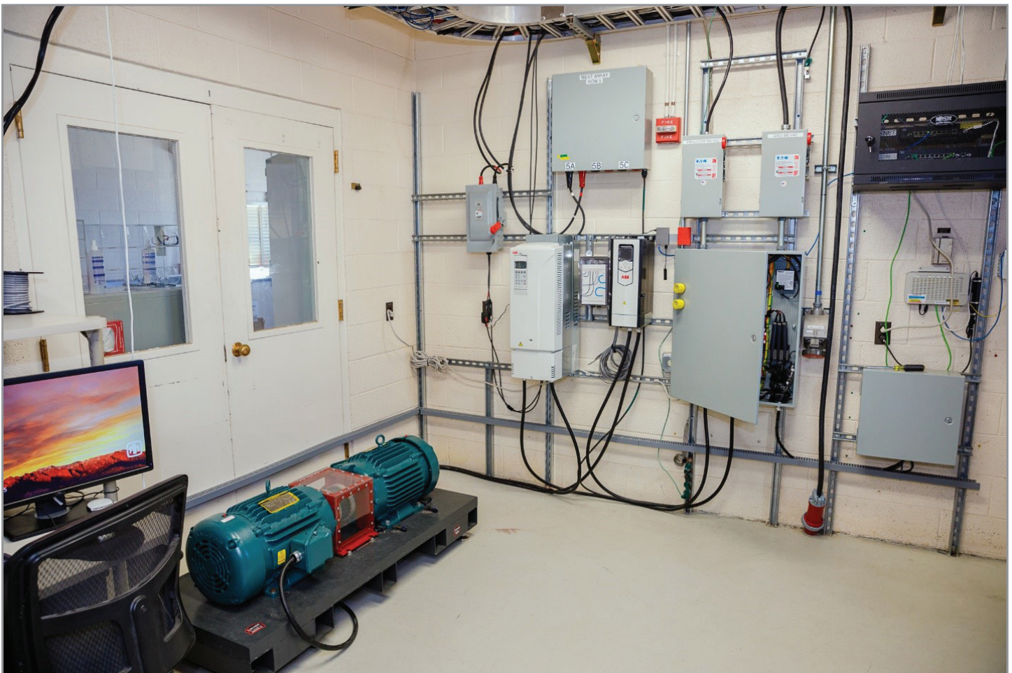
Power hardware-in-the-loop installed at the DETL Image Credit: Sandia, Bret David Latter
