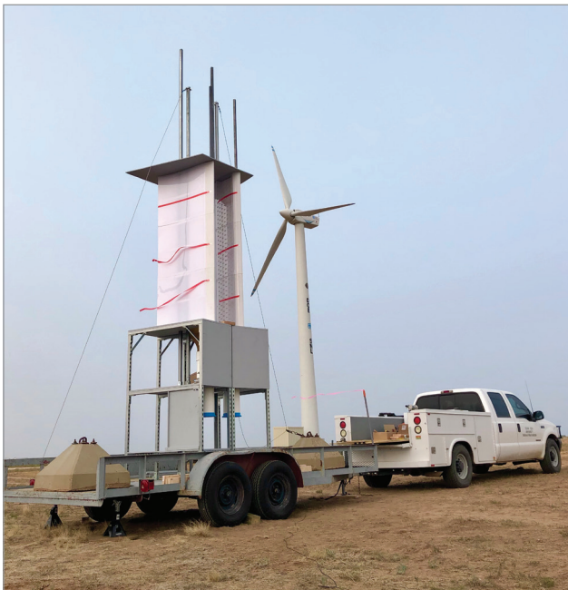
Pilot-scale testing AeroMINE at SWiFT. Image credit: Rebecca Gustaf
