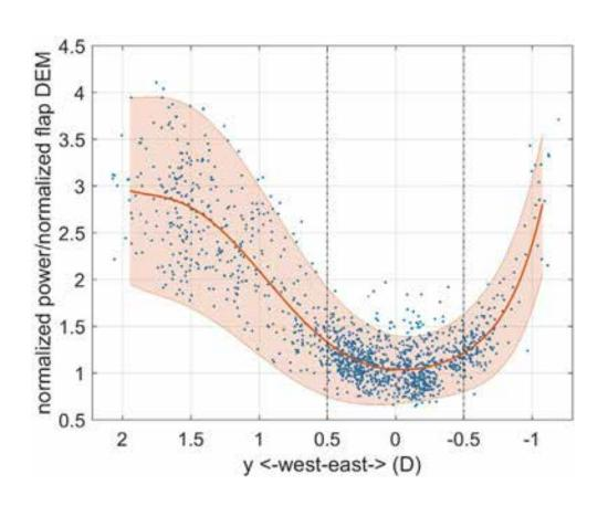
Metric created from the ratio of normalized power by normalized flap DEM fatigue damage
