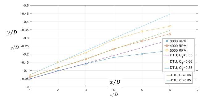
Comparison of measured wake deflection center  $y_c(x)$  for  $\omega$ =3000, 4000, and 5000 RPM at yaw angle of  $\gamma = 20^\circ$  with wake deflection given by DTU wake deflection model.
