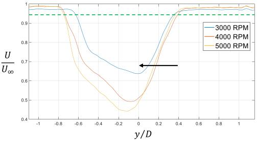
Comparison of normalized mean stream-wise velocity  $(U/U_{\infty})$  profile in the hub-height horizontal plane at x/D=3 for yaw angle  $\Upsilon$ =20°.
