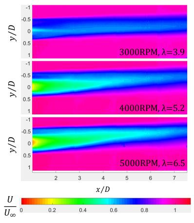
Contours of the normalized mean streamwise velocity  $(U/U_{\infty})$  in the horizontal plane at hub height for several RPM at  $\Upsilon = 20^{\circ}$ .
