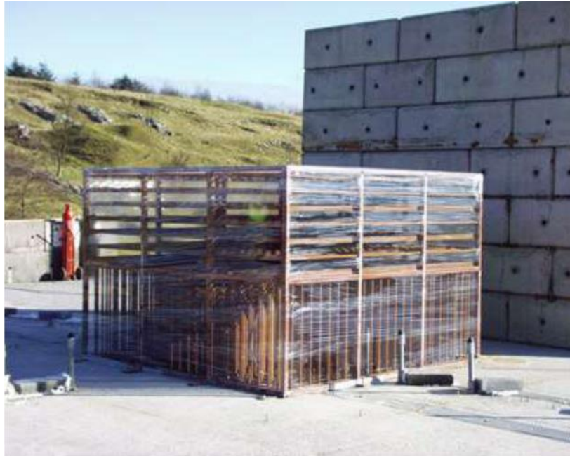
Figure 68: Congestion region or grid where gas was filled then ignited (from [123])
