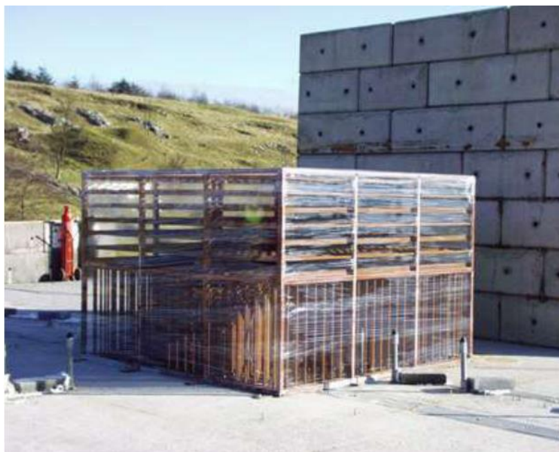
Figure 29: Congestion region or grid where gas was filled then ignited (from [123])
