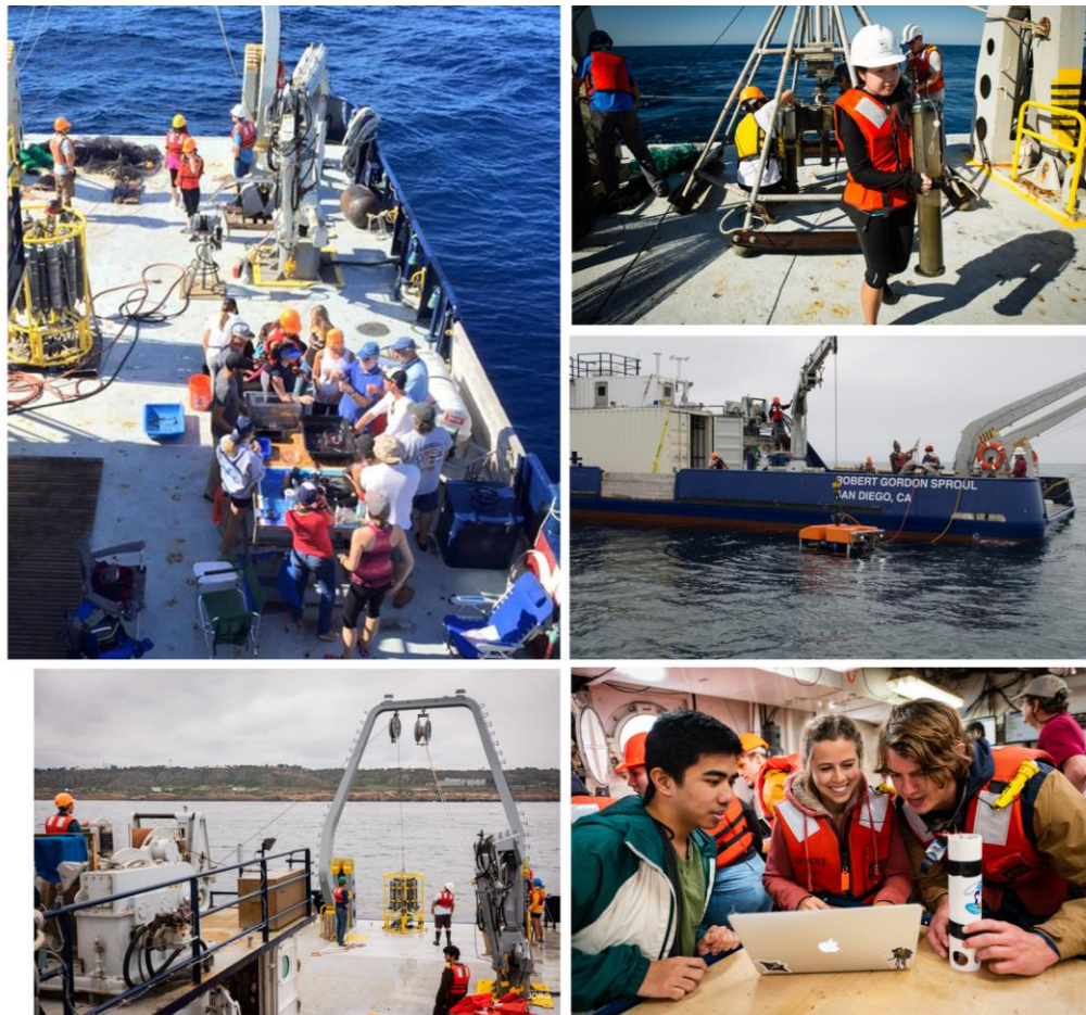
Figure 2: Research and instructional activities onboard the R/V Robert Gordon Sproul . Clockwise from top left: A marine biology class sorts through the contents of a successful Isaacs-Kidd Midwater Trawl; a fresh seabed sample from a multicore is carried by a student across the deck to the laboratory; scientists and technicians deploying a Remotely-Operated Vehicle (ROV) to investigate deep-sea ecosystems associated with a natural seabed methane vent offshore La Jolla; students in the ship's Electronics Laboratory download data from a sensor (that they built in class) that had been lowered to the seabed; a group of students prepares to deploy a Conductivity-Temperature-Depth (CTD) profiling rosette. Photo Credits: The Scripps Institution of Oceanography.
