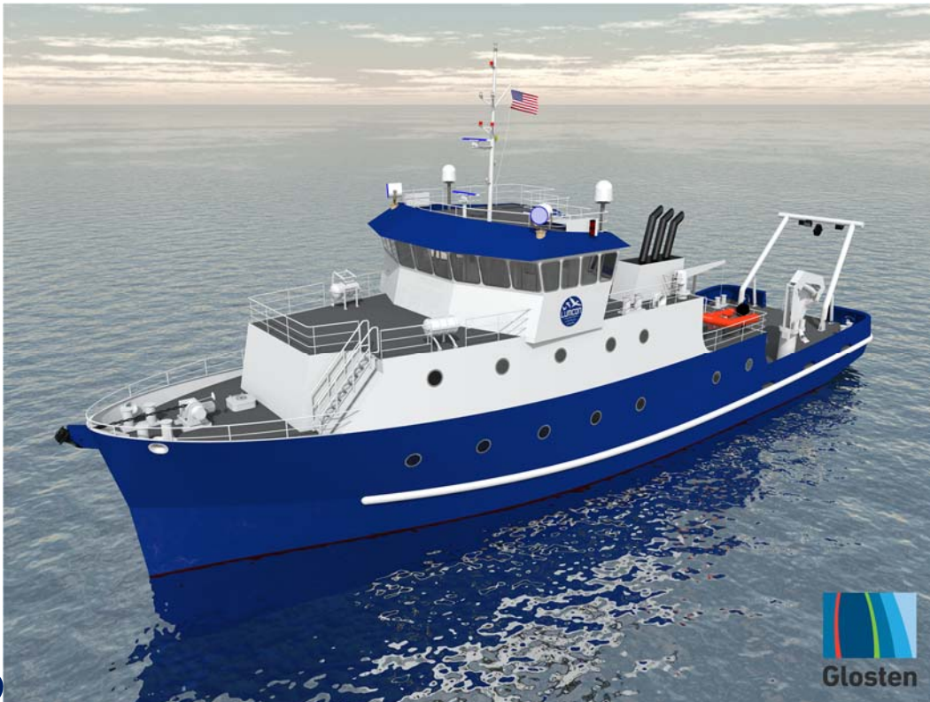
Figure 1 SRV baseline hull - 125-foot research vessel concept
