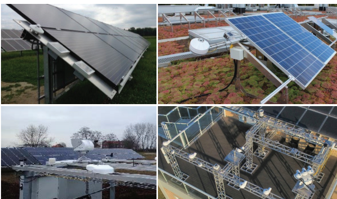
Figure 2. Images of irradiance sensors at three field sites: (clockwise from top left) POA pyranometer and reference cells on baseline system in Vermont, USA; POA pyranometer and PV-modules in Halle, Germany; GHI and DNI sensors in Köthen, Germany; irradiance sensors in Florianopolis, Brazil; (above) albedometer in Vermont.
