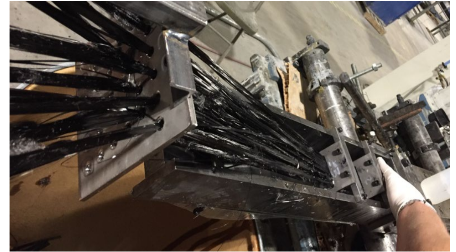
CFTF material being dipped through resin and pulled through the pultrusion die.
