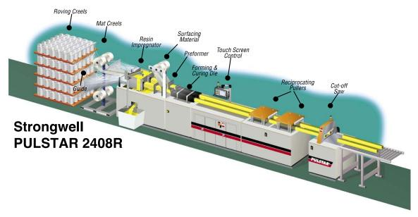
Figure 2-1. Example pultrusion manufacturing process.
