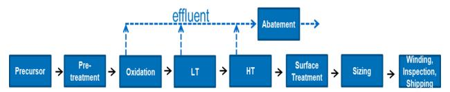
Figure 2-11. Sequential major processing steps of carbon fiber manufacturing.
