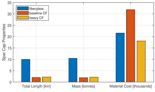
Figure 4-3. Land-based turbine optimal solution spar cap properties.
