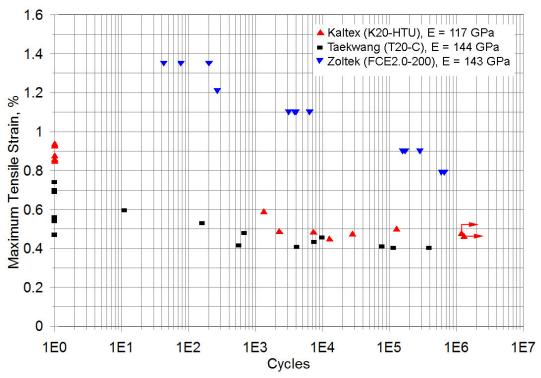
Figure 2-10. Fatigue test comparison of the study materials, R=0.1 (Zoltek in commercial pultrusion (V<sub>F</sub>=62%), CFTF materials in aligned strand infusion (V<sub>F</sub>~50%)).
