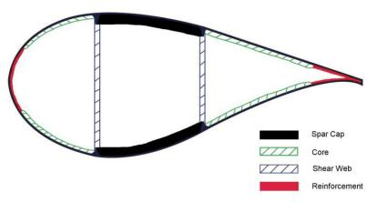
Figure 1-6. Wind turbine blade sectional drawing with region identification.
