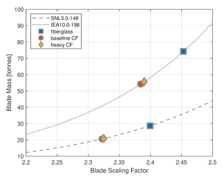
Figure 5-1. Blade mass scaling (*mass=length* <sup>scaling factor</sup>) utilizing the three study materials (dashed lines show traditional blade mass scaling; markers show mass results from this study).
