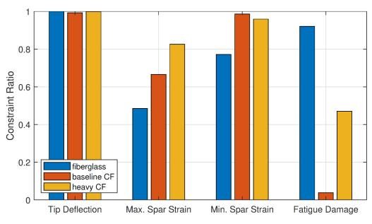
Figure 4-1. Land-based turbine optimal solution constraint values.
