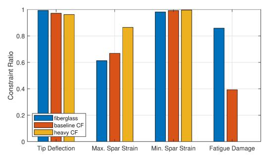
Figure 4-4. Offshore turbine optimal solution constraint values (nearly infinite fatigue life prediction for the heavy tow textile carbon fiber).
