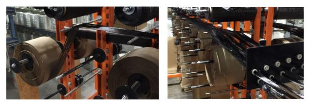
Figure 2-8. CFTF tows mounted to spindles and traversing guides for pultrusion.
