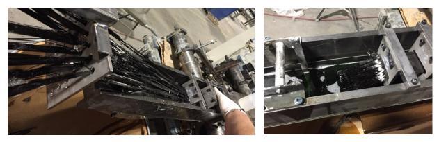
Figure 2-9. CFTF material being dipped through resin and pulled through the pultrusion die.
