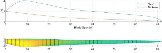
Figure 3-1. Top view and chord and thickness profiles for the SNL 3MW reference blade.
