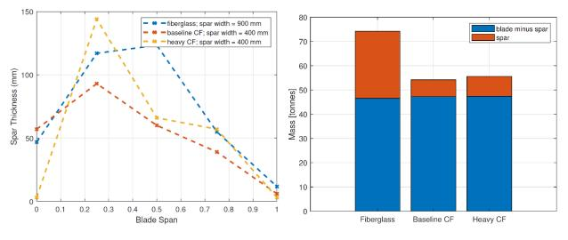
(a) Spar cap thickness profile comparison (b) Spar cap and blade mass comparison
