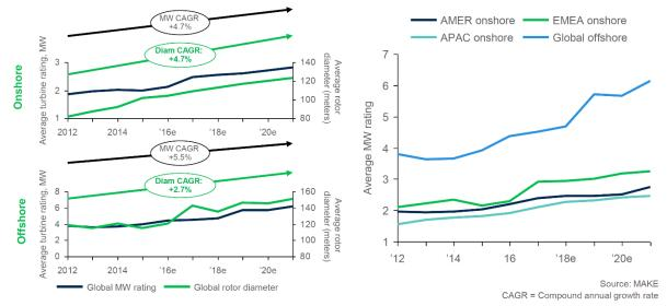
Figure 1-1. Global trends for wind turbine power rating and diameter increase.
