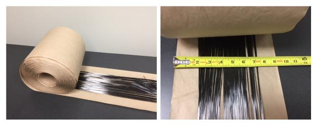
Figure 2-6. Example of initial heavy-tow CFTF material winding.
