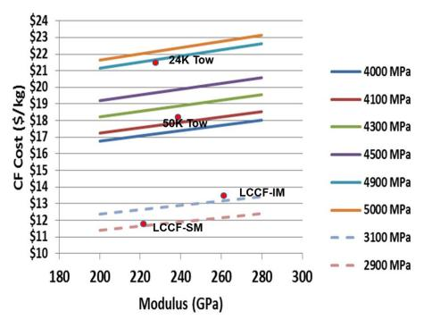
Figure 2-14. Carbon fiber cost sensitivity to its mechanical properties.
