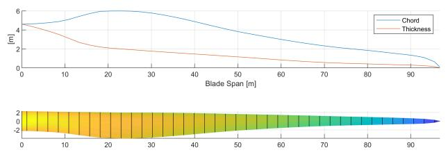
Figure 3-2. Top view and chord and thickness profiles for the IEA 10 MW reference blade.
