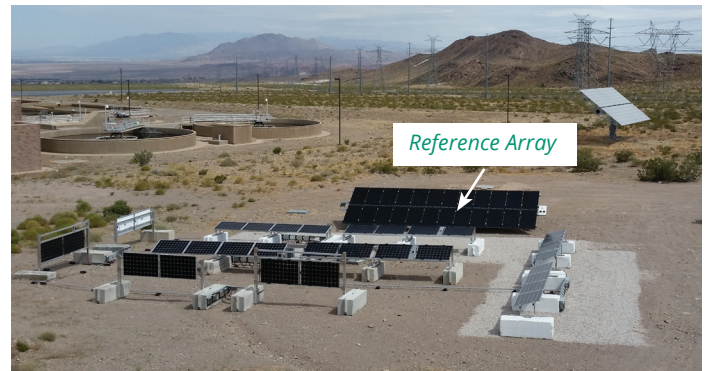
Roof-top view of the Nevada RTC, with fixed-tilt PV systems in the center; open-racking to accommodate new installations to the right; and CPV trackers to the rear.
