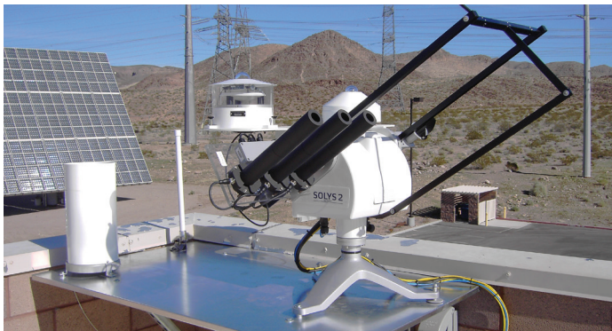
GPS solar tracker and irradiance sensors at the Nevada RTC collect high-fidelity irradiance data, including GHI, DHI and DNI and spectral composition, at a frequency of every 5 seconds.
