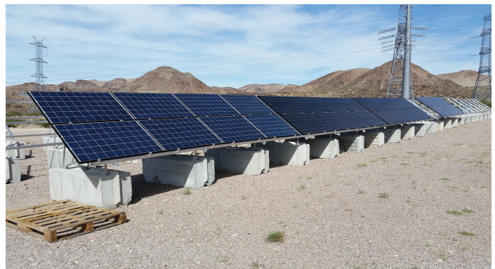
Energy output and other performance data from multiple module technologies, such as the ones depicted above, are collected and analyzed by Sandia, and shared with the industry partners.
