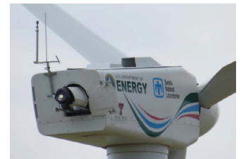
SpinnerLIDAR mounted in nacelle at SWiFT for downwind wake measurements.
