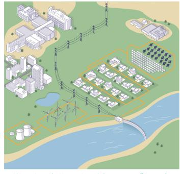
Within a microgrid, ESS asset size and placement can affect overall system performance, return on investment, and interactions with the larger grid. Sandia capabilities can help a utility optimize its choices.
