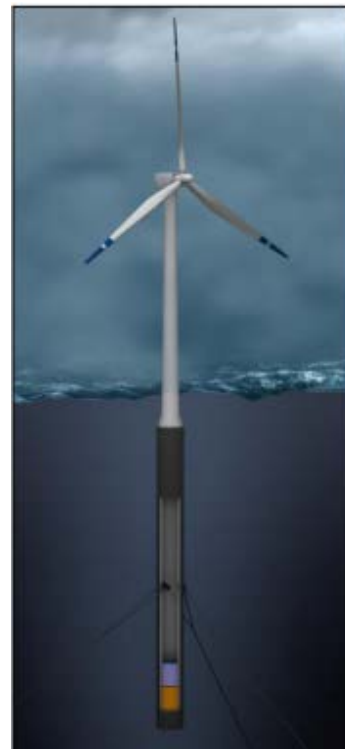
Figure 93. a) WindFloat Semi-Submersible (31) and b) Hywind Spar (32).
