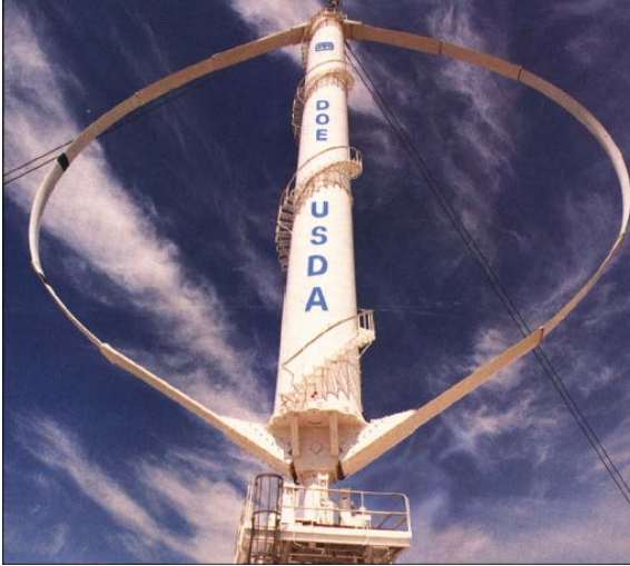
Figure 8. The Sandia 34 meter VAWT Testbed.
