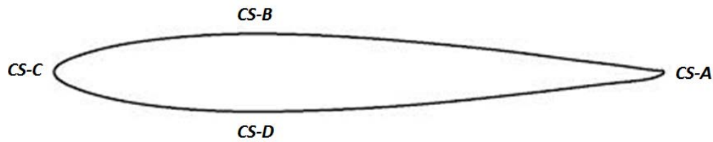
Figure 83. Cross-sectional locations examined for strain extrema.
