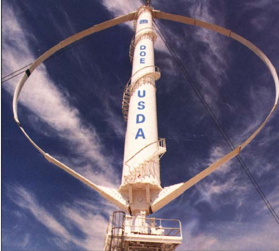
Figure 38. The Sandia 34 meter VAWT Testbed.
