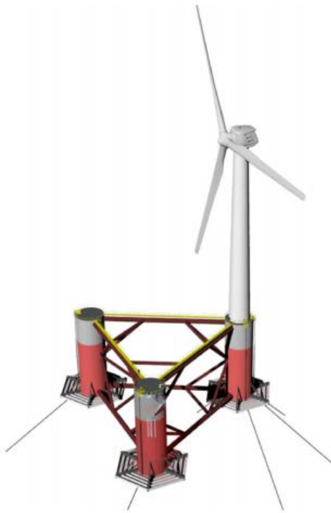
Figure 93. a) WindFloat Semi-Submersible (31) and b) Hywind Spar (32).
