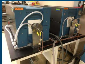
High temperature corrosion furnaces (setup / used in FY17 corrosion tests)
