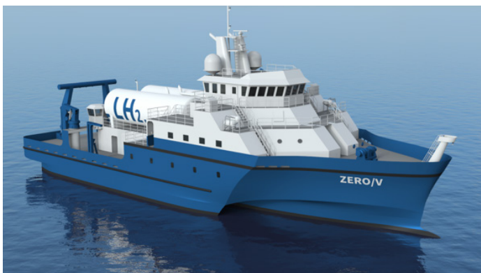
Figure 1: Renderings of the Zero-V zero-emission hydrogen fuel cell research vessel.
