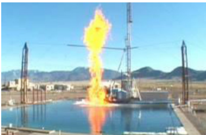
Figure 10: A 10-m diameter LNG pool fire from the Sandia Phoenix Tests. Figure reproduced from Reference 56.
