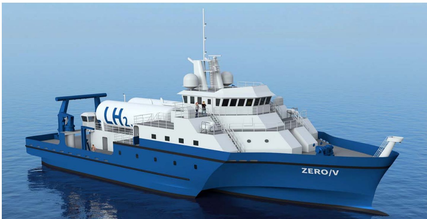
Figure 13(a): Side rendering of the Zero-V zero-emission hydrogen fuel cell research vessel.
