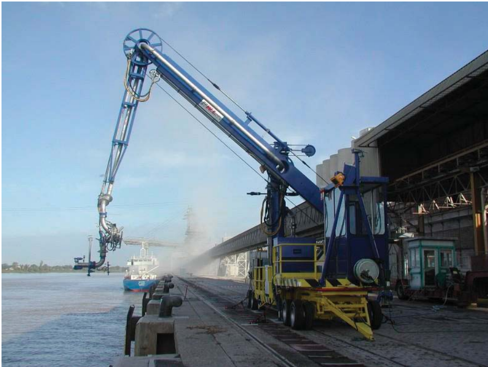
Figure 16 Mobile marine loading arm (Wiese Europe)
