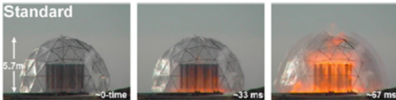
Figure 8: High-speed optical video images of hydrogen combustion for a 30% hydrogen/air mixture, ignited with a 40 J spark. Figure reproduced from Reference 48.
