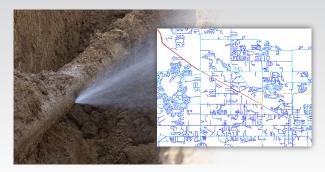
The Sandia-developed Water Network Tool for Resilience (WNTR) software simulates and analyzes the resilience of water distribution networks. Increasing resilience to hazards such as pipe breaks due to aging infrastructure, natural disasters, or terrorist attacks is essential to improving water security.
