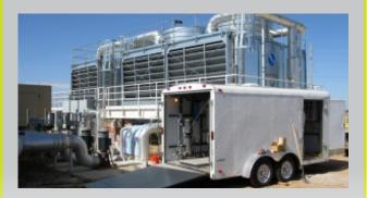
Sandia has conducted field-scale pilot tests for water treatment technologies of both coal-bed methane produced water and cooling tower water, shown above.
