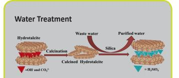
Examples of novel water treatment technologies developed at Sandia include the R&D100 award-winning highpermeability biomimetic membranes, graphene oxide membranes, fouling resistant treatments for commercial RO membranes, and designer sorbants, such as easily recyclable hydrotalcite for silica removal, shown above.
