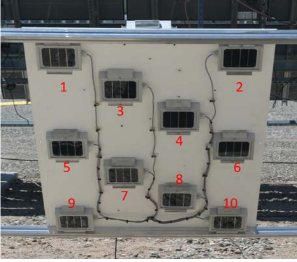
Fig. 1. Movable sensor array for high spatial resolution measurements of rear-surface irradiance.
