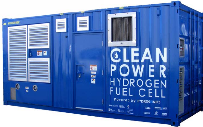
Figure ES-1: The maritime fuel cell generator, with integrated hydrogen storage, PEM fuel cell power generation, and power inverter equipment can power up to 10 reefers with a total rated output of 100 kW at 240 VAC.
