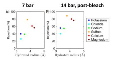
Treat-to-need rejection of salts in cooling tower blowdown water.
