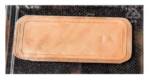
Following month-long rejection tests, no biofilm growth is observed on the GO/polymer membranes
