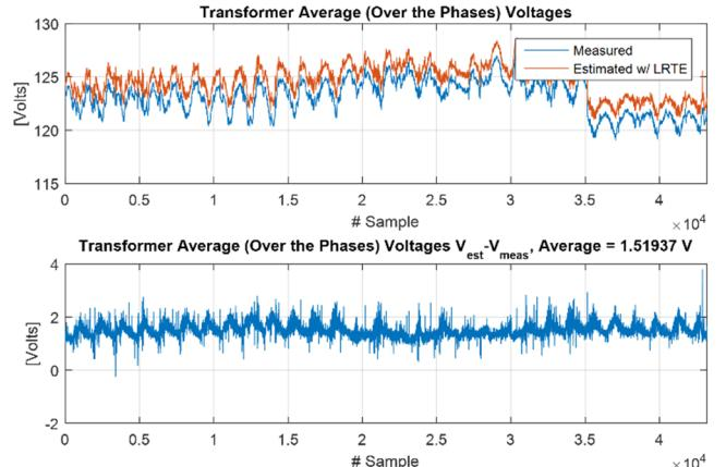
Fig. 10 LRTE estimated transformer voltage measurement offset
