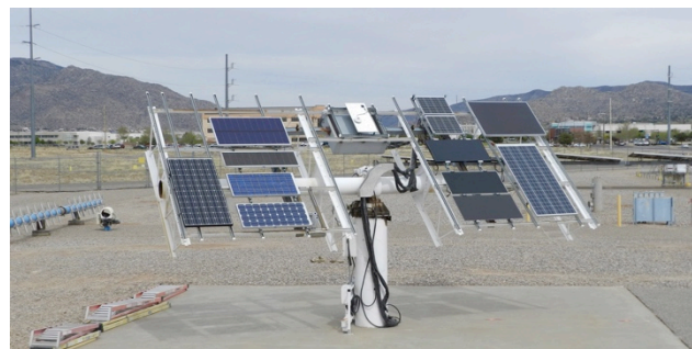
Fig. 1. Modules under test on a two-axis tracker at Sandia
