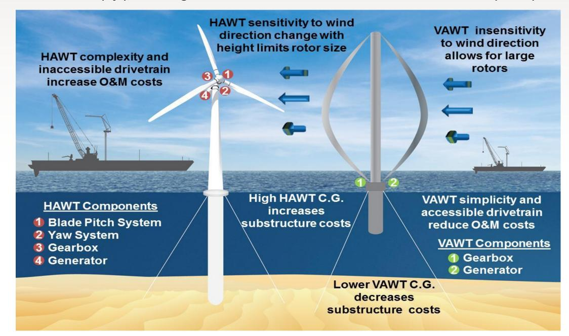
Vertical axis wind turbines (VAWTs) represent a deep-water solution with inherent advantages over horizontal axis wind turbines (HAWTs). For example, placement of the drivetrain at the base of the tower lowers the vertical center of gravity and improves accessibility of drivetrain components for installation and O&M, major cost drivers positively impacted by VAWTs.
