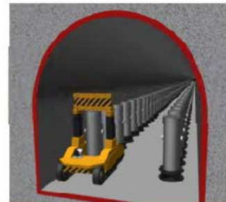
A. Initial Emplacement Phase of storage casks In CARE uses standard technology which can be tele-operated
