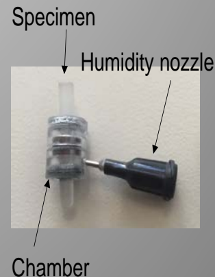
Prototype of corrosion chamber – made of PMMA
