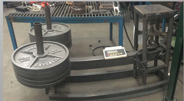
d) Photograph showing implant testing machine at CSM
