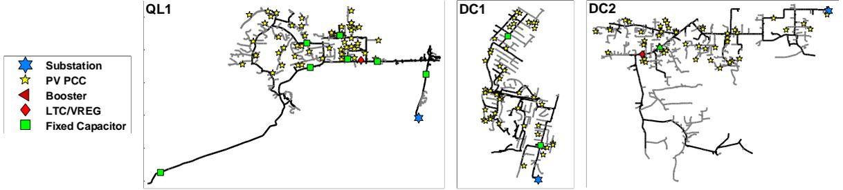
Figure 3. Topologies of the full circuit models of feeder QL1 (left), DC1 (middle), and DC2 (right)
