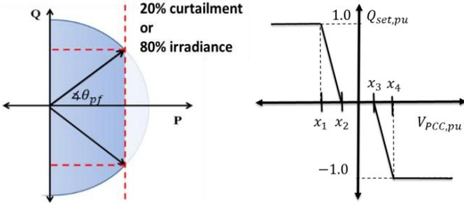
Figure 2. (left) Assumed relationship between real power output and reactive power available to PV inverter. (right) Volt/Var droop curve used for reactive power support.
