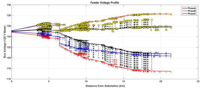
Figure 4. Feeder voltage profile at minimum load without PV and with PV, represented as yellow stars.
