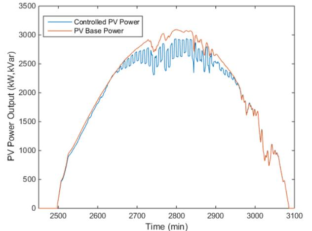
Figure 8. Daytime inverter power output under 5-minute dispatch of sensitivity-based curtailment compared to the base power output.
