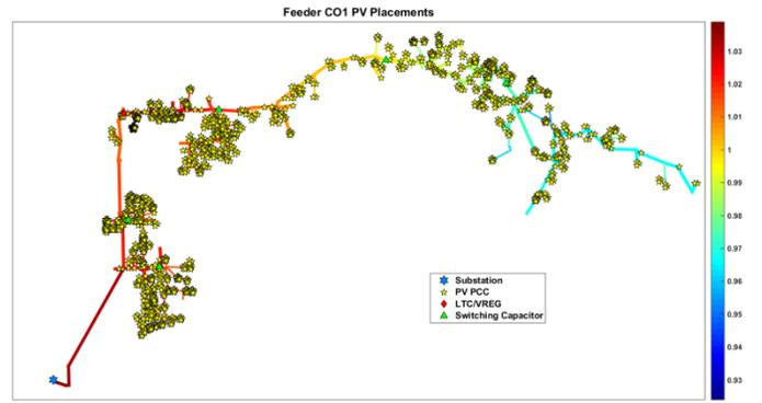
Figure 3. Map of feeder CO1 with PV placements indicated and lines colored by per-unit voltage.
