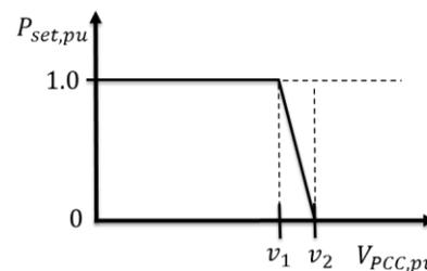
Figure 1. Volt/Watt droop curve used for local PV power curtailment.
