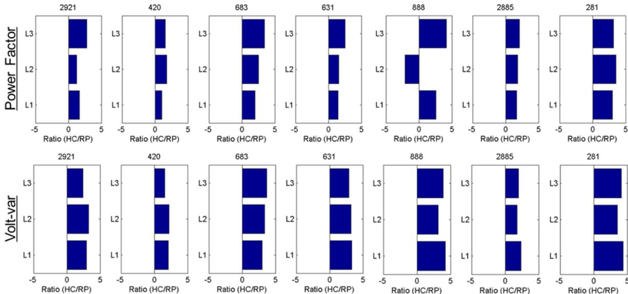
Fig. 5. Ratio of hosting capacity to reactive power for each study feeder and each method to determine the settings.
