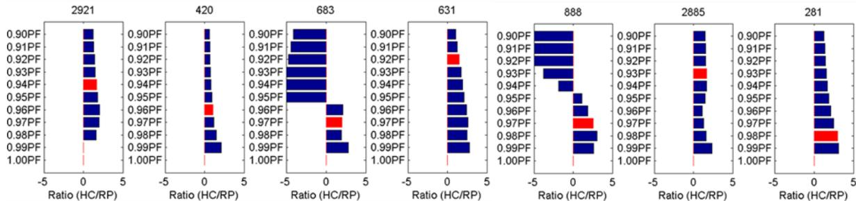
Fig. 6. Ratio of benefit to impact for power factor brute force analysis. The Level 1 power factor settings are highlighted in red.
