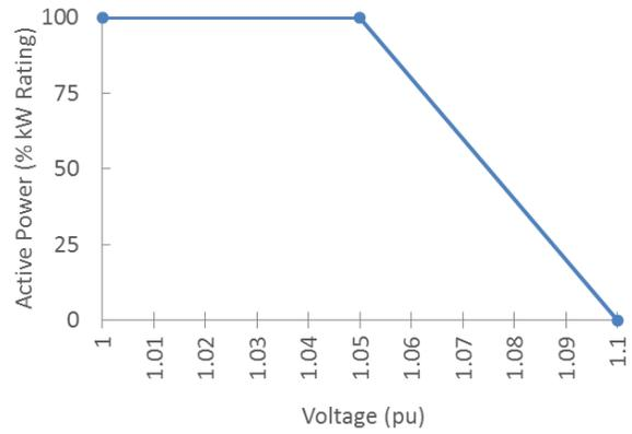
Fig. 3. Level 1 volt-watt setting.
