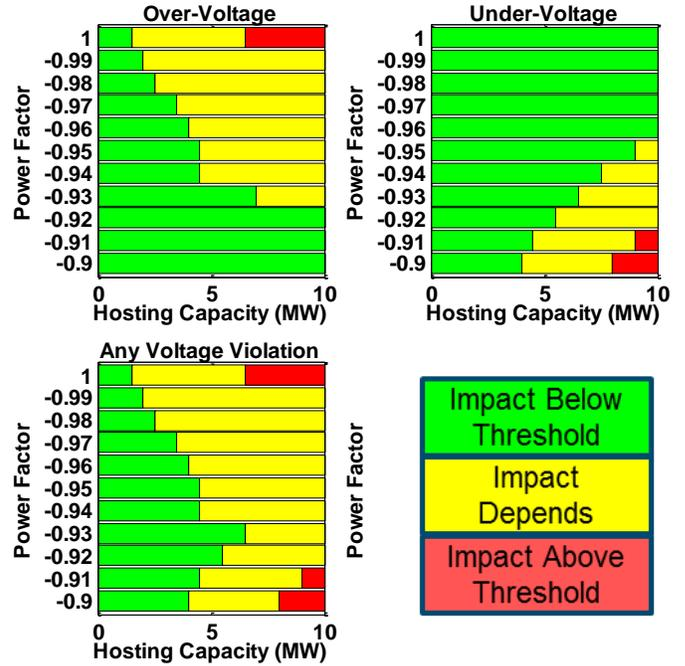
Fig. 1. Hosting capacity analysis for feeder 631 at various inductive power factors.
