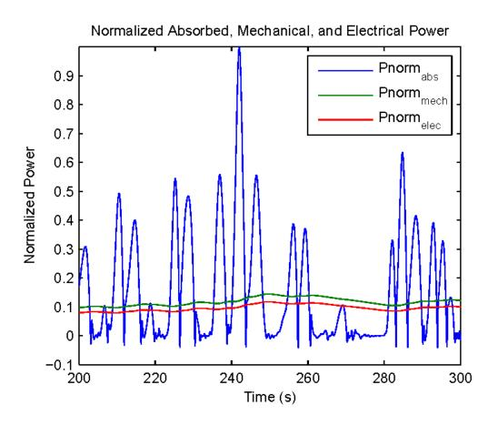
$P_{abs}$  is the power absorbed at the piston  $P_{mech}$  is the power at the axle connecting the motor and generator  $P_{elec}$  is the electrical power at the output of the generator
