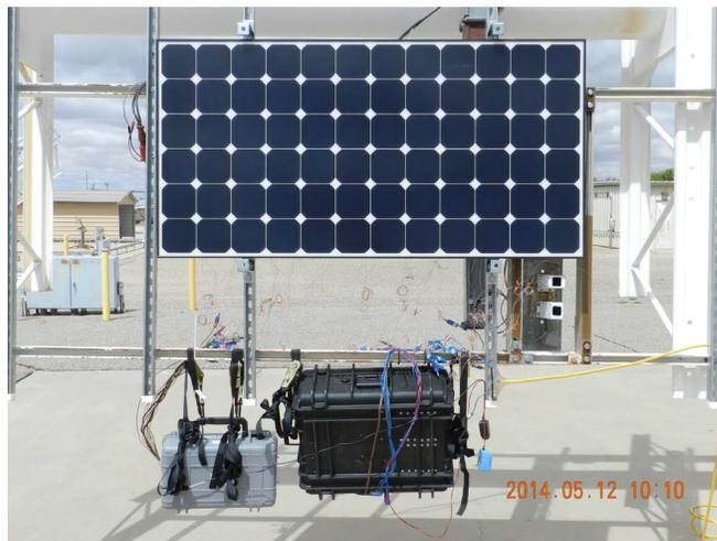
Fig. 1. 72 cell module mounted on tracker with data loggers.
