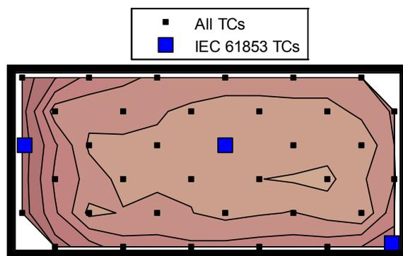
Fig. 2. Thermocouple locations on the 72 cell module.
