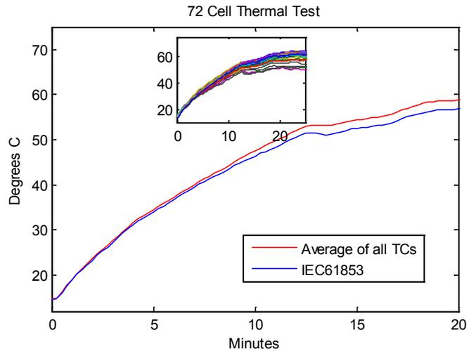
Fig. 3. Temperature measurements for the 72 cell module.
