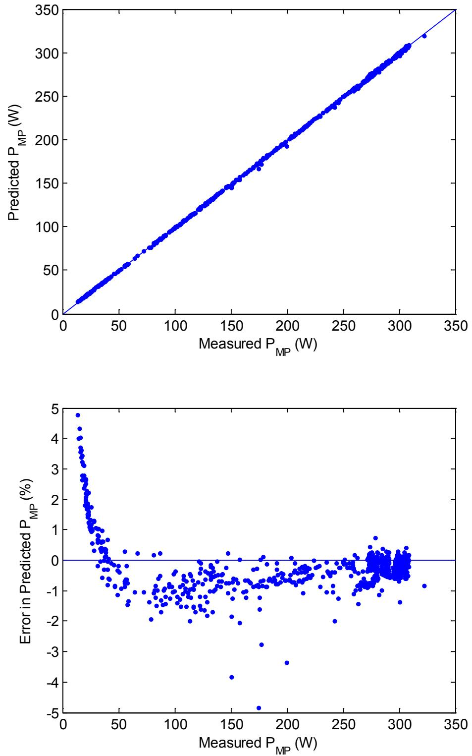
**Figure 17. Predicted vs. measured power and relative error in predicted power.**
