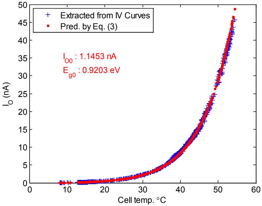
**Figure 9. Determination of  $I_{O0}$  and  $E_{g0}$ .**
