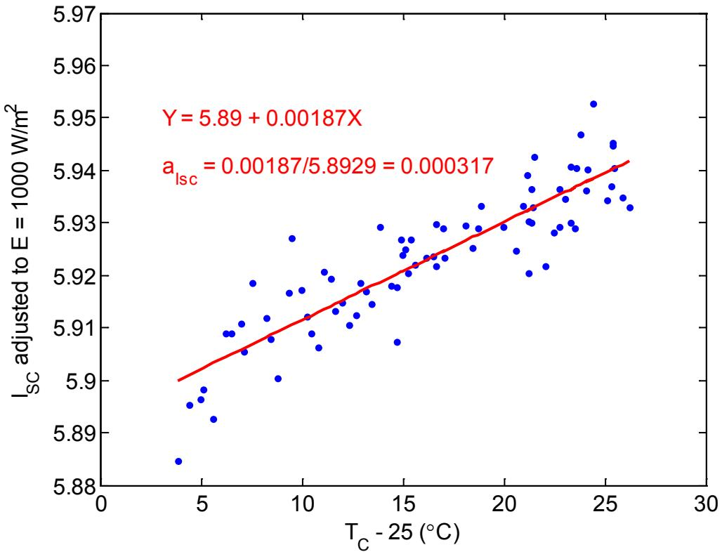
**Figure 5. Example of determination of  $\alpha_{Isc}$ .**
