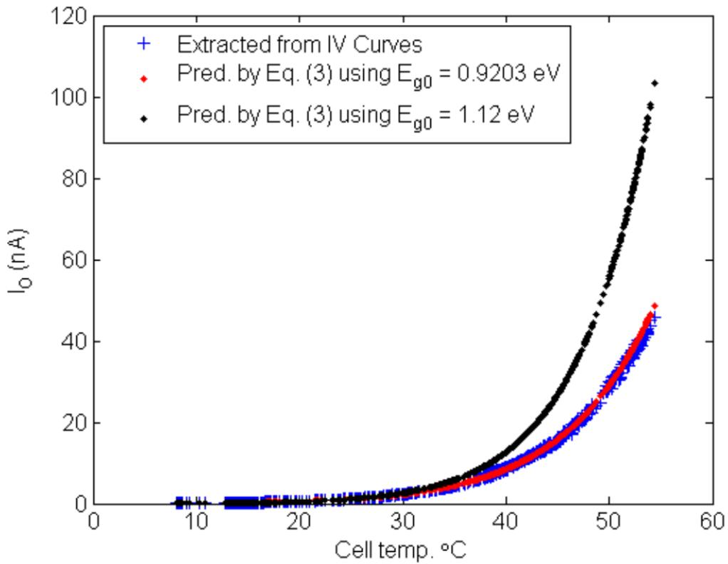
**Figure 10. Comparison of extracted values for  $I_o$  with values computed using theoretical and empirical values for  $E_{g0}$ .**
