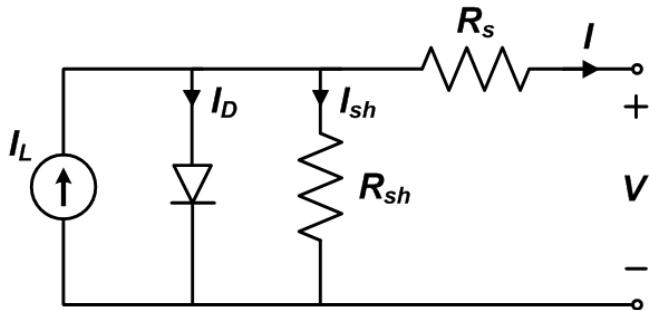
Figure 1. Single diode equivalent circuit for a PV cell or module.
