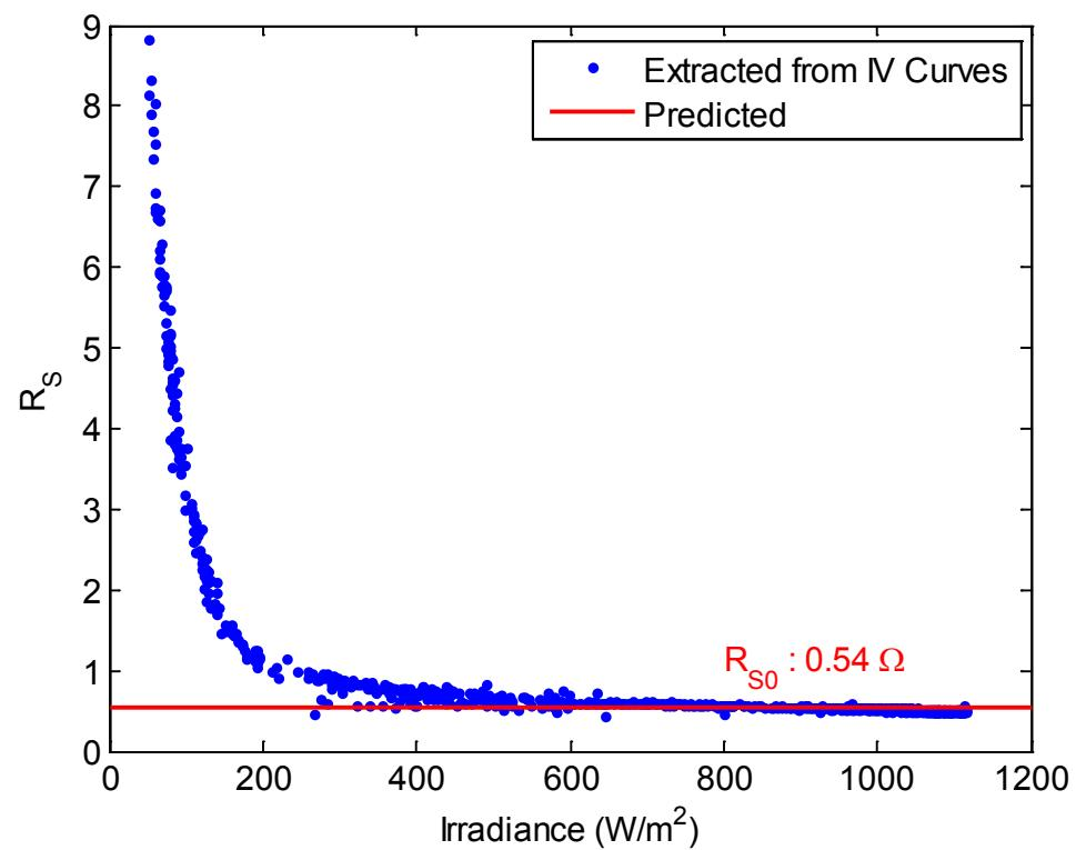
Figure 11. Determination of  $R_{SH0}$  (top) and  $R_{S0}$  (bottom).
