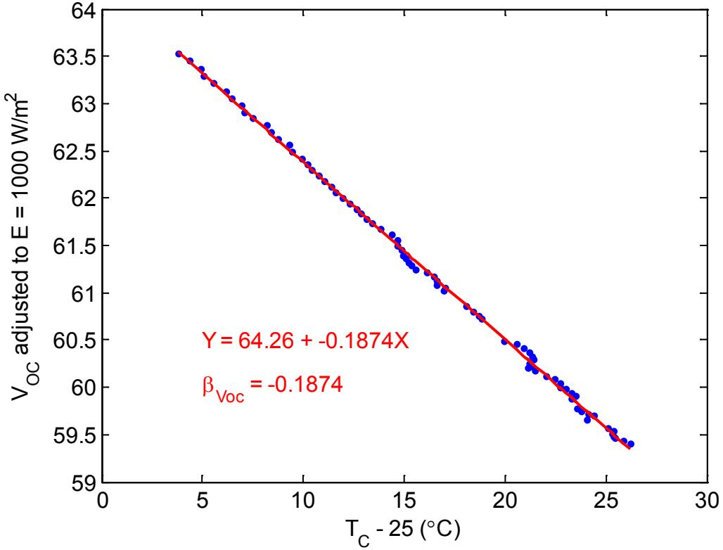
**Figure 4. Example of determination of  $\beta_{Voc}$ .**
