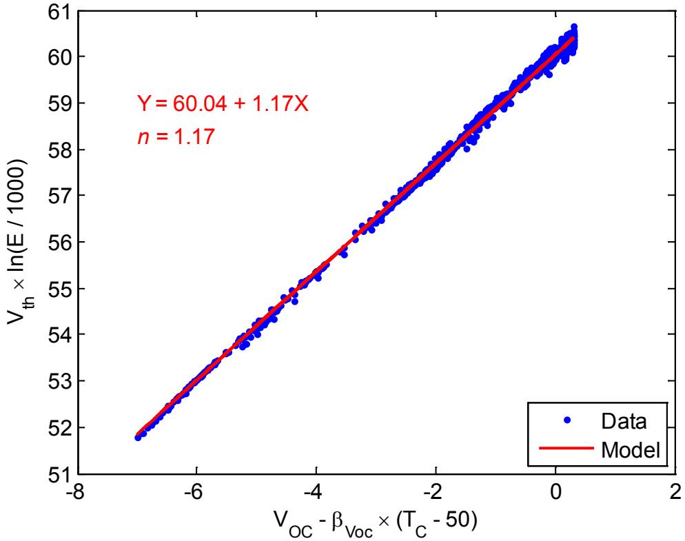
**Figure 6. Example of determination of  $n$ .**
