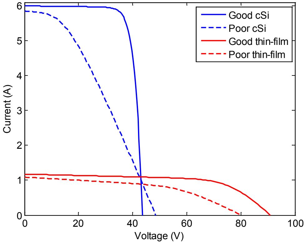
**Figure 12. I-V Curves at STC for simulated modules.**
