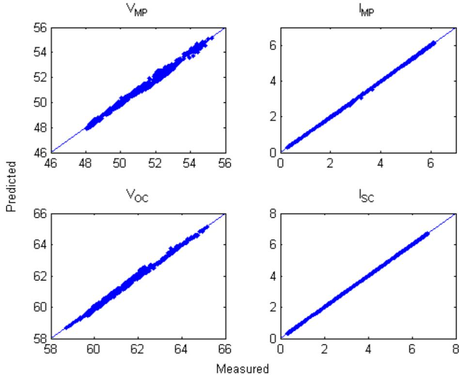
**Figure 15. Predicted vs. measured voltage and current.**
