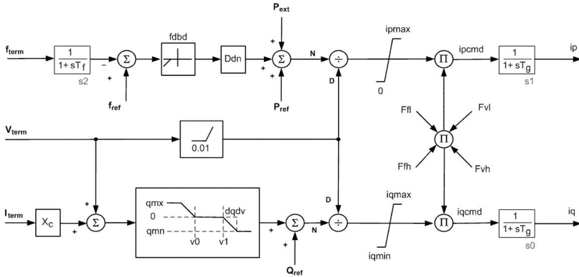
Figure 6. Distributed PV system model.
