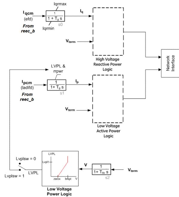
Figure 2. Renewable energy generator/converter module.
