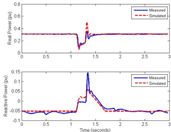
Figure 5. Model validation example for a PV inverter.
