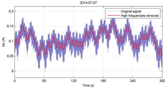
Fig. 7. DC current signal with and without high-frequency content
