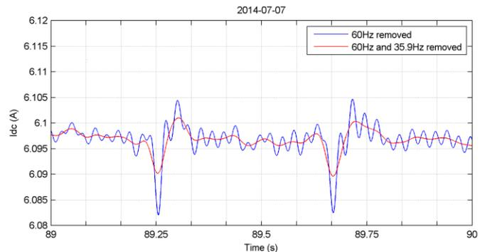
Fig. 6. DC current signal with 60 Hz and 35.9 Hz harmonics removed (close-up)
