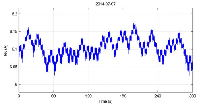
Fig. 5. DC current signal with 60 Hz harmonics removed
