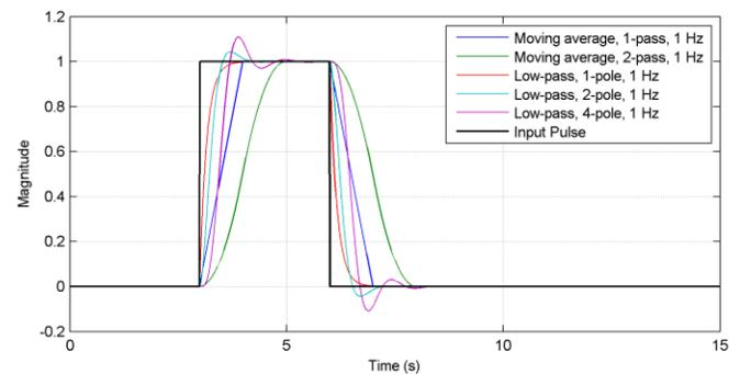
Fig. 2. Step response of several filter types
