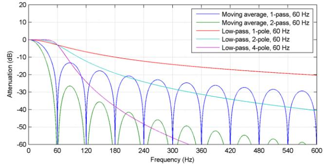
Fig. 1. Frequency response of several filter types
