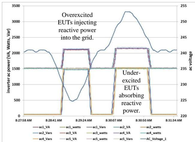
Fig. 5. Volt-VAr evaluations conducted on five inverters.
