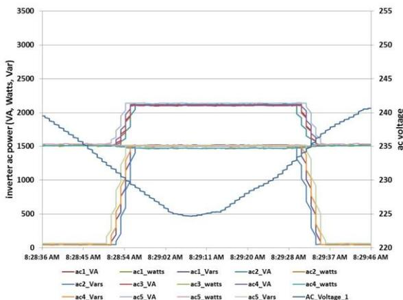
Fig. 6. Detailed five-inverter volt-VAr test results.
