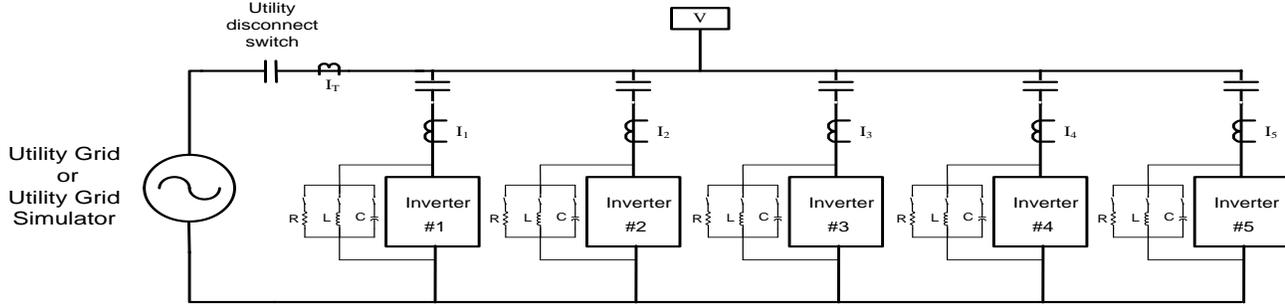
Fig. 2. Single or multi-inverter test configuration.
