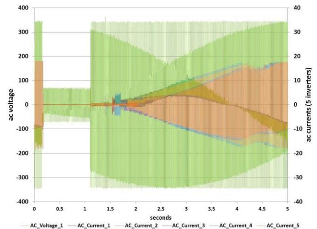
Fig. 4. Voltage < 50% of nominal ride through (5-inverter configuration).
