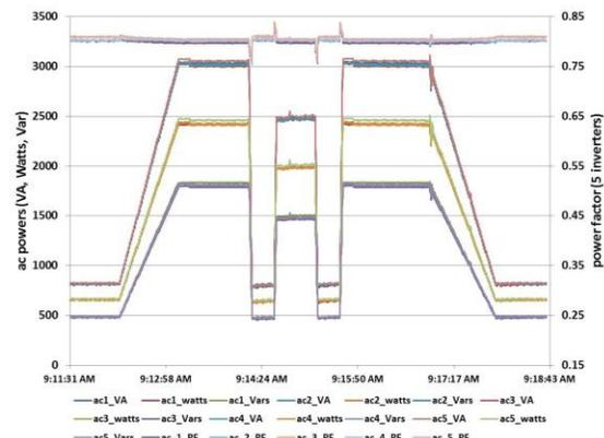
Fig. 7. PF evaluation with varying dc/ac power.
