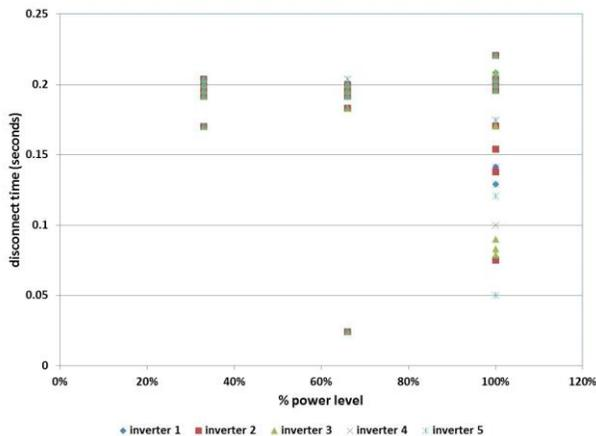
Fig. 11. Unintentional islanding test results with five inverters.
