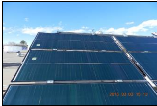
Fig. 5. Opaque partial shade applied to module surface.
