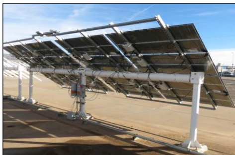
Fig. 2. Photograph of back side of testbed showing I-V tracers connected to string of 16 fixed-tilt modules.
