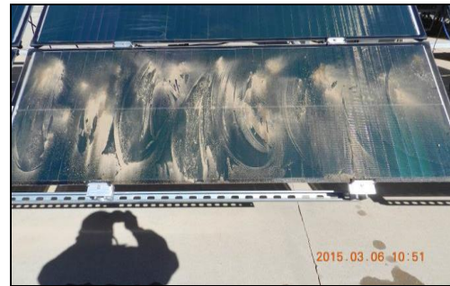
Fig. 8. Module shown with applied dirt for soiling example.
