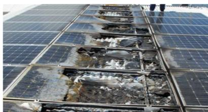
Damage resulting from an arc fault in the PV array. If left undetected, loss of life could result in addition to property damage.
