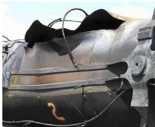
Figure 7-3. Car with Thermal Tear.
