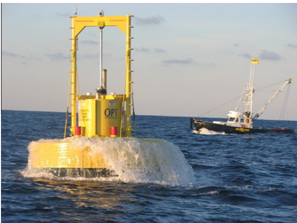
Fig. 1. A prototype of OPT's PowerBuoy wave energy generation system. NREL PIX # 17114.
