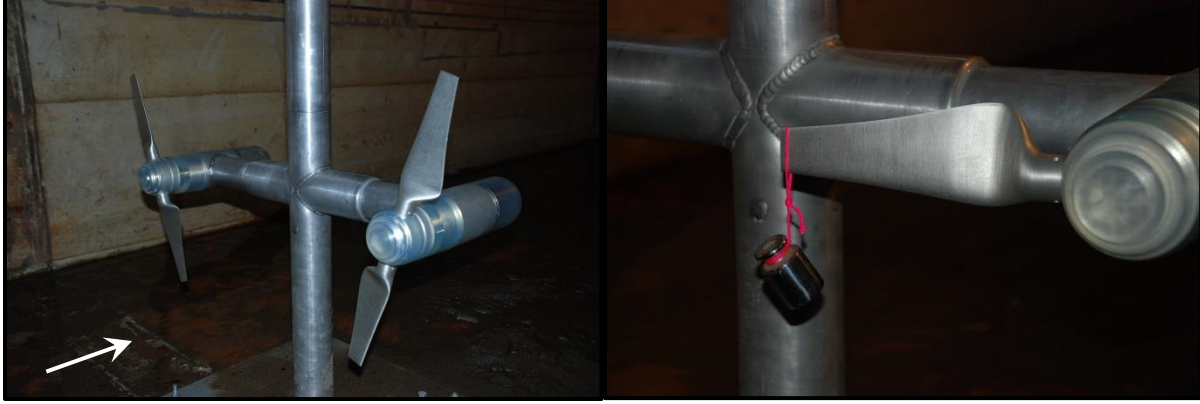
Figure 3: Photos of the RM1 dual-rotor model in the SAFL Main Channel (left) and during torque sensor calibration (right) performed by applying known forces to the rotor and torque sensor.
