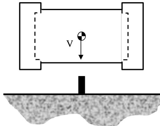
1 m drop onto 15 cm steel bar
