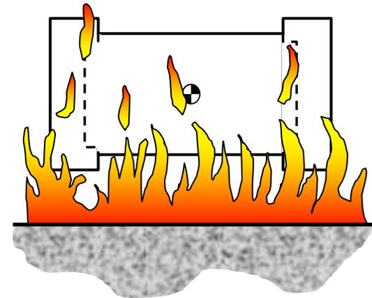
800 °C fully engulfing fire for 30 minutes
