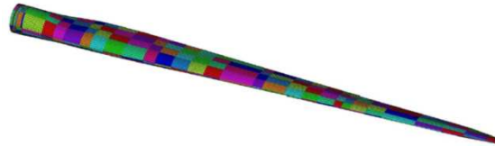
Figure 1. ANSYS finite element mesh for the 5-MW blade model
