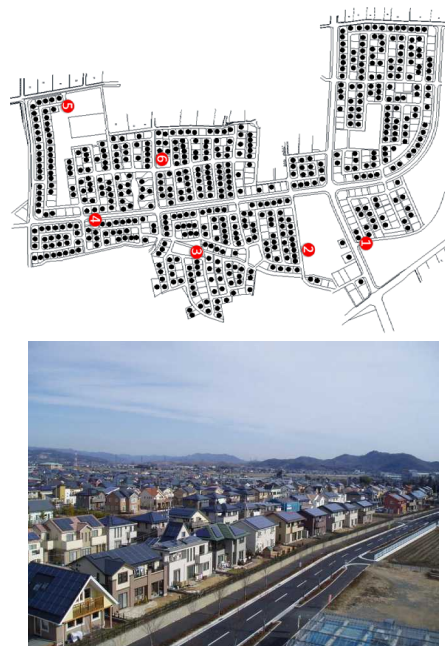
Fig. 1. Layout of homes with PV (black dots) in the neighborhood and a photograph of Pal Town in Ota City. [2]
