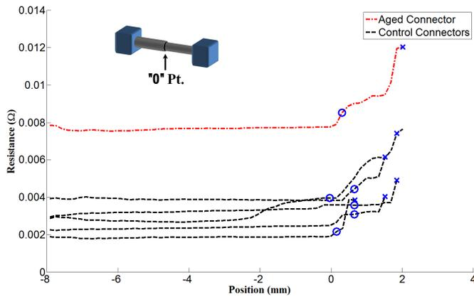
Fig.7. Measured resistance plotted as a function of translational stage position during arc fault experiment for manufacturer B. The five dark solid lines represent five new connector pins and the dashed red line represents a corroded connector. The blue circles indicate the location of the first detected arc. The blue “x” shows the location where a sustained arc began to occur.
