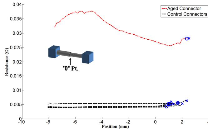
Fig. 8. Measured resistance plotted as a function of translational stage position during arc fault experiment for manufacturer C. The five dark solid lines represent five new connector pins and the dashed red line represents a corroded connector. The blue circles indicate the location of the first detected arc. The blue “x” shows the location where a sustained arc began to occur.
