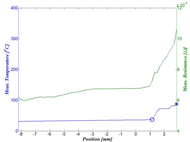
Fig.9. Measured connector temperature and resistance plotted as a function of translational stage position during arc fault experiment. The blue “o” indicates the onset of the first observable spark event, while the “x” indicates the onset of sustained arcing.
