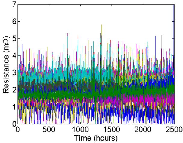
Fig. 5. Contact resistance data for connectors exposed to the elements in a high-desert outdoor environment. The measurements are noisier than the laboratory measurements due to temperature cycles. The results will be used to help infer connector lifetime from accelerated test results.
