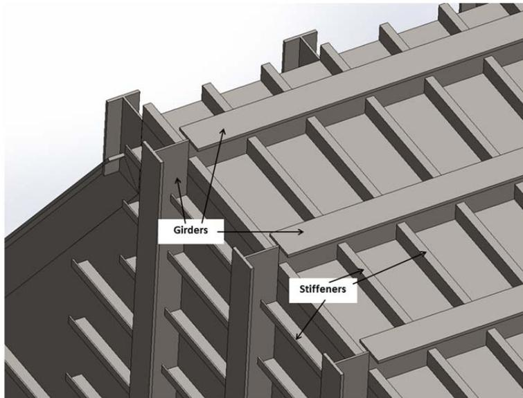
**Figure 2: Illustration of girders and stiffeners used in Re Vision design.**
