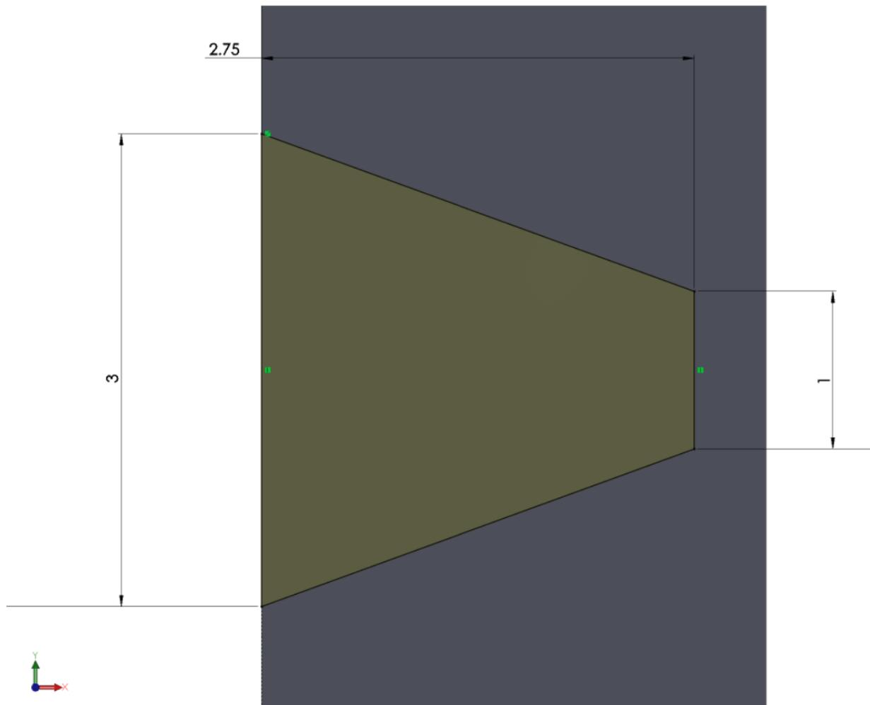
**Figure 11: Dimensions of intermediate support plate in meters.**
