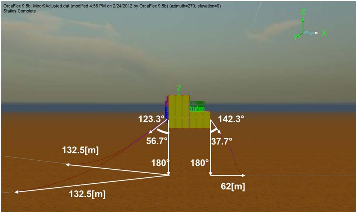
**Figure 5: Side view of mooring line configuration in Orcaflex.**
