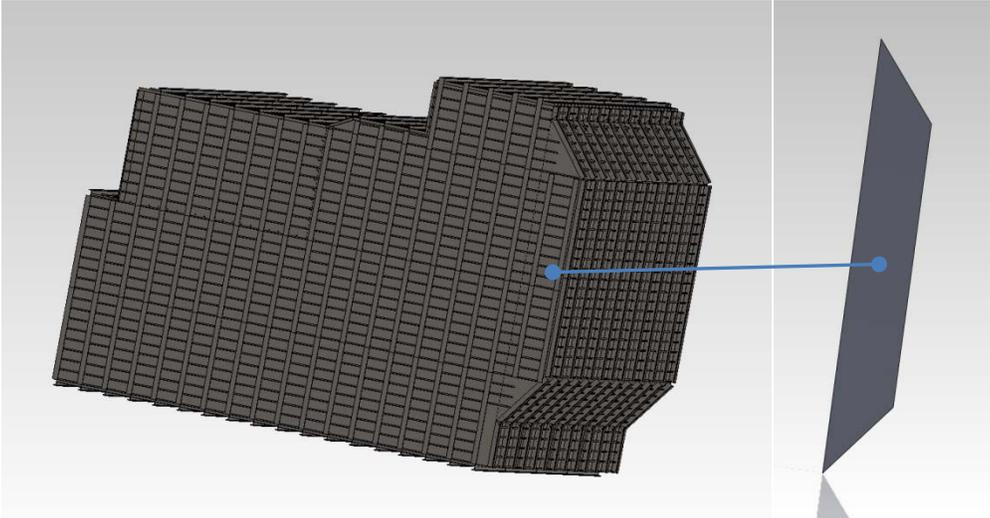
**Figure 6: OWC buoyancy chamber plate where mooring attachment point is located.**
