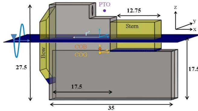
**Figure 14: Model of the OWC describing dimensions, locations of principal components, locations of the COB and COG, and identifying coordinate systems.**
