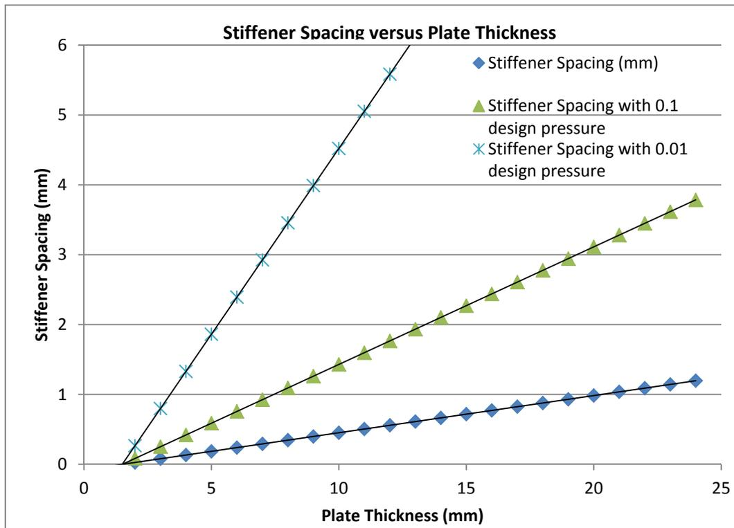
**Figure 1: DNV relationship between stiffener spacing and plate thickness. The blue triangles illustrate the relationship used by Re Vision Consulting. The green triangles and blue stars illustrate how this relationship changes with the design pressure (values chosen specifically in relationship to RM3 reference case discussed above).**
