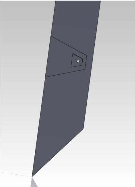
**Figure 7: Additional plates to support the maximum mooring load. Attachment point also shown.**
