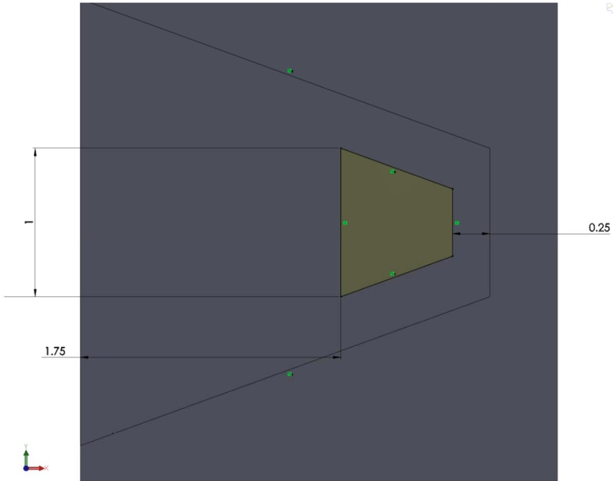
**Figure 12: Dimensions of outer support plate in meters.**
