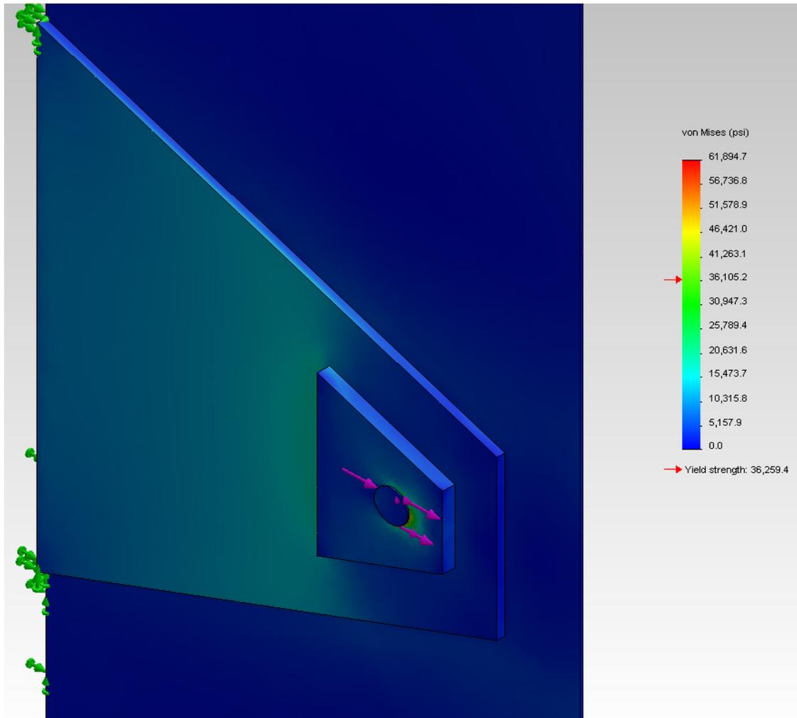
**Figure 10: Simulation results for a 2320 kN mooring load.**
