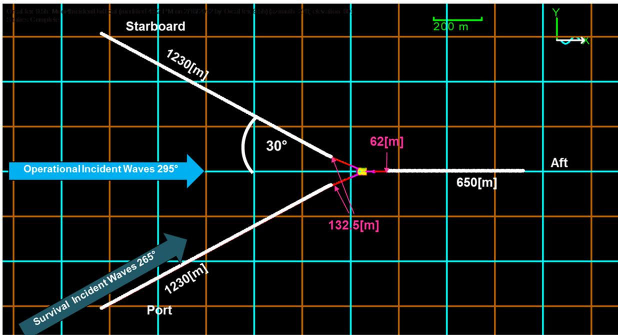
Figure 4: Plan view of mooring line configuration in Orcaflex.
