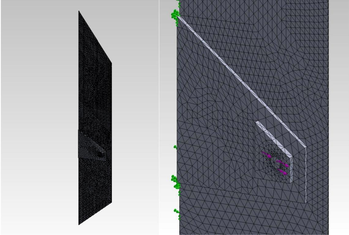
**Figure 9: Full and enlarged view for the buoyancy plate simulation with mesh shown.**
