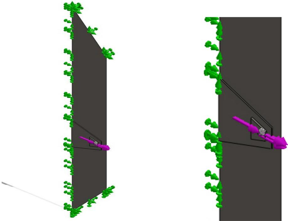
**Figure 8: Full and enlarged view for the buoyancy plate with fixed and load bearing locations shown.**
