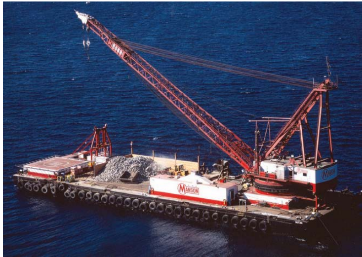
Figure 3-17. Example of a 500-tonne capacity crane barge.
