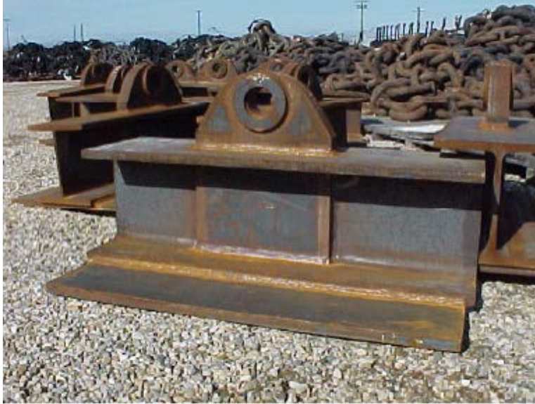
Figure 4-17. Plate anchor with pad eye.
