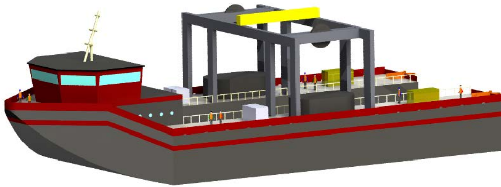
Figure 3-21. Custom DP-2 vessel with moonpool.
