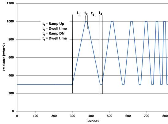
Figure 10. Irradiance profile for small & medium irradiance intensities
