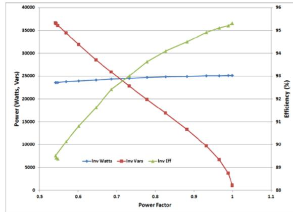
Figure 6. Inverter efficiency vs power factor during volt/var
