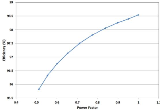
Figure 8. Inverter efficiency during commanded power factor operation
