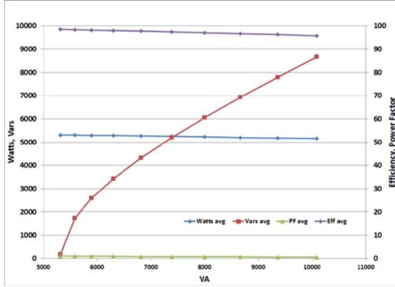
Figure 7. Inverter power delivered during commanded power factor
