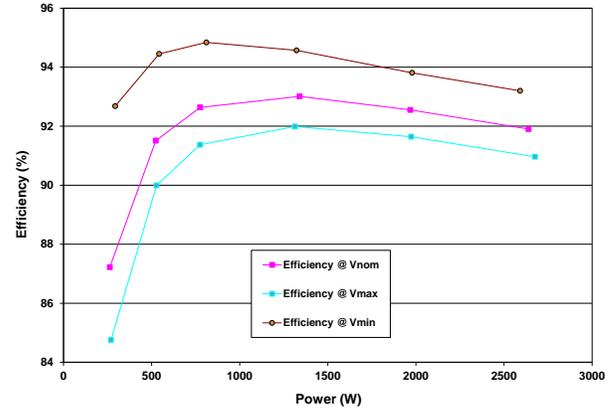
Figure 9. Efficiency curves using parameters from Table 1
