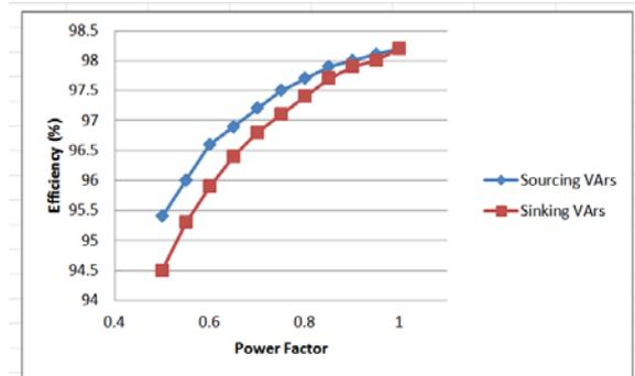
Figure 3. Efficiencies of a modeled 250 kW PV inverter as a function of power factor, while sinking or sourcing VAr.
