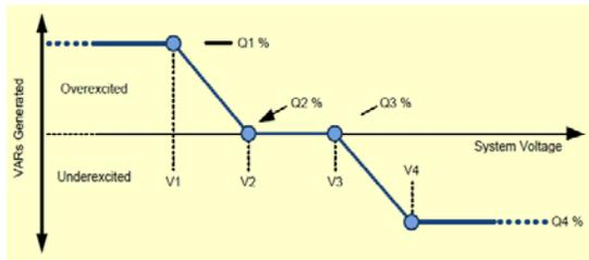
Figure 4. V1–V4: the adjustable voltage percentages and Q1–Q4: the adjustable reactive power percentages
