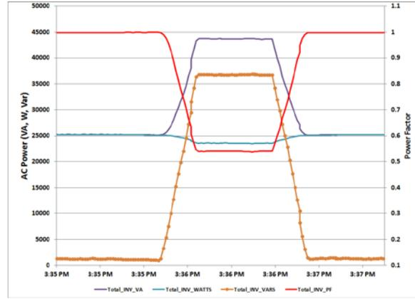
Figure 5. Inverter power delivery during implementation of volt/VAr advanced inverter function VV11
