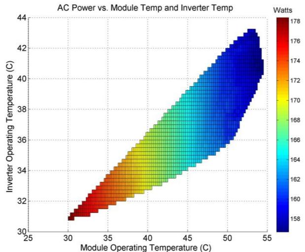
Fig. 3. Irradiance-corrected AC power as a function of module and inverter temperature.
