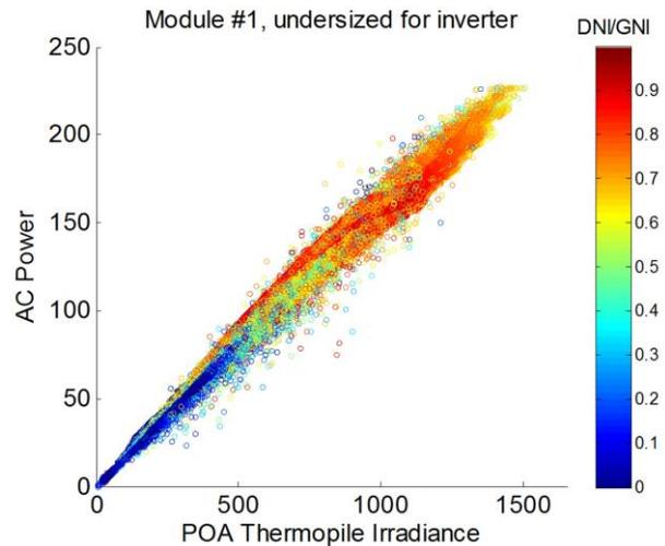
Fig. 8. System 1 measured AC power with irradiance, colored for DNI/GNI ratio.
