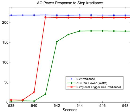
Fig. 1. AC power response to step change in irradiance.
