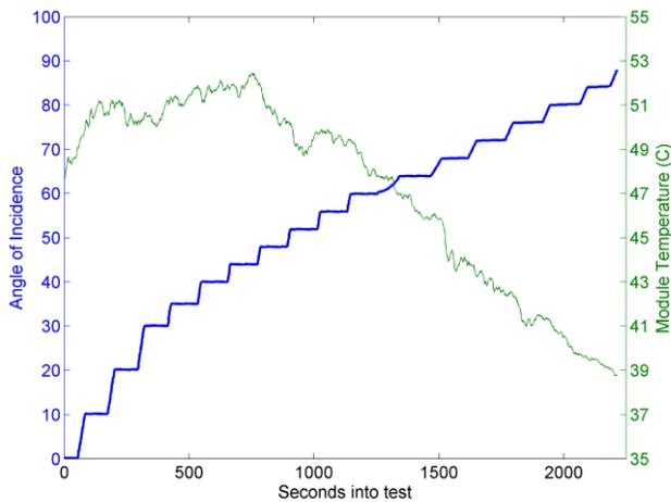
Fig. 5. AOI and module temperature during incident angle testing.
