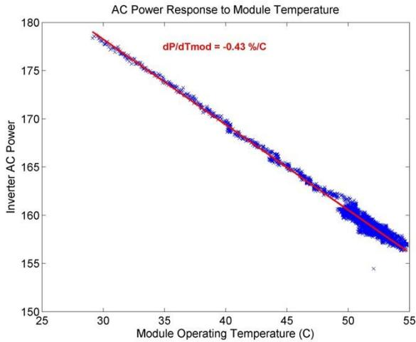
Fig. 4. Irradiance-corrected AC Power as a function of module temperature.
