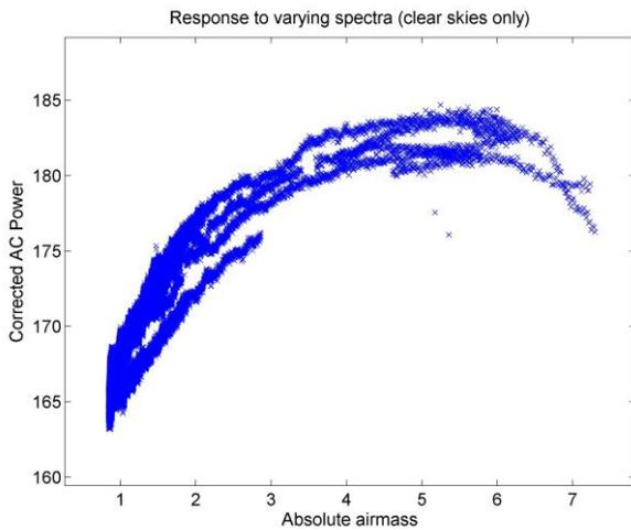
Fig. 7. Temperature and irradiance corrected AC power as a function of airmass.
