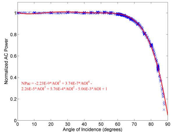
Fig. 6. System response to incident angle, fit with a polynomial.
