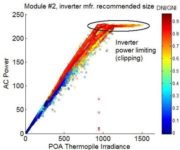
Fig. 9. System 2 measured AC power with irradiance, colored for DNI/GNI ratio.
